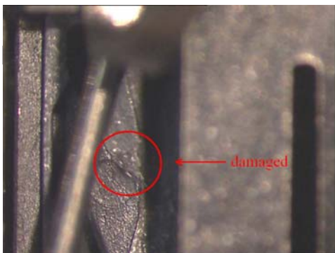
Lock mechanism damaged
