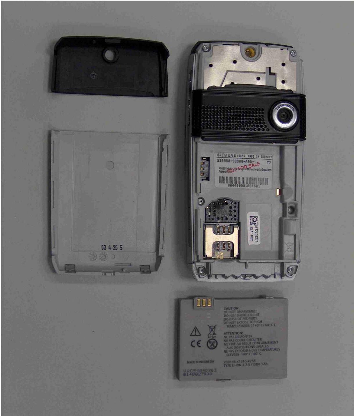
Figure 1 SXG75 Open Battery Cover (Final label: See extra exhibit)
