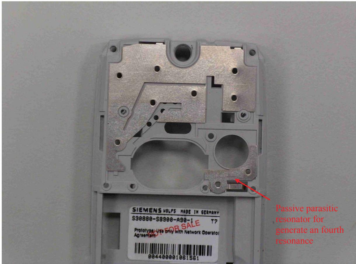
Passive parasitic resonator for generate an fourth resonance
