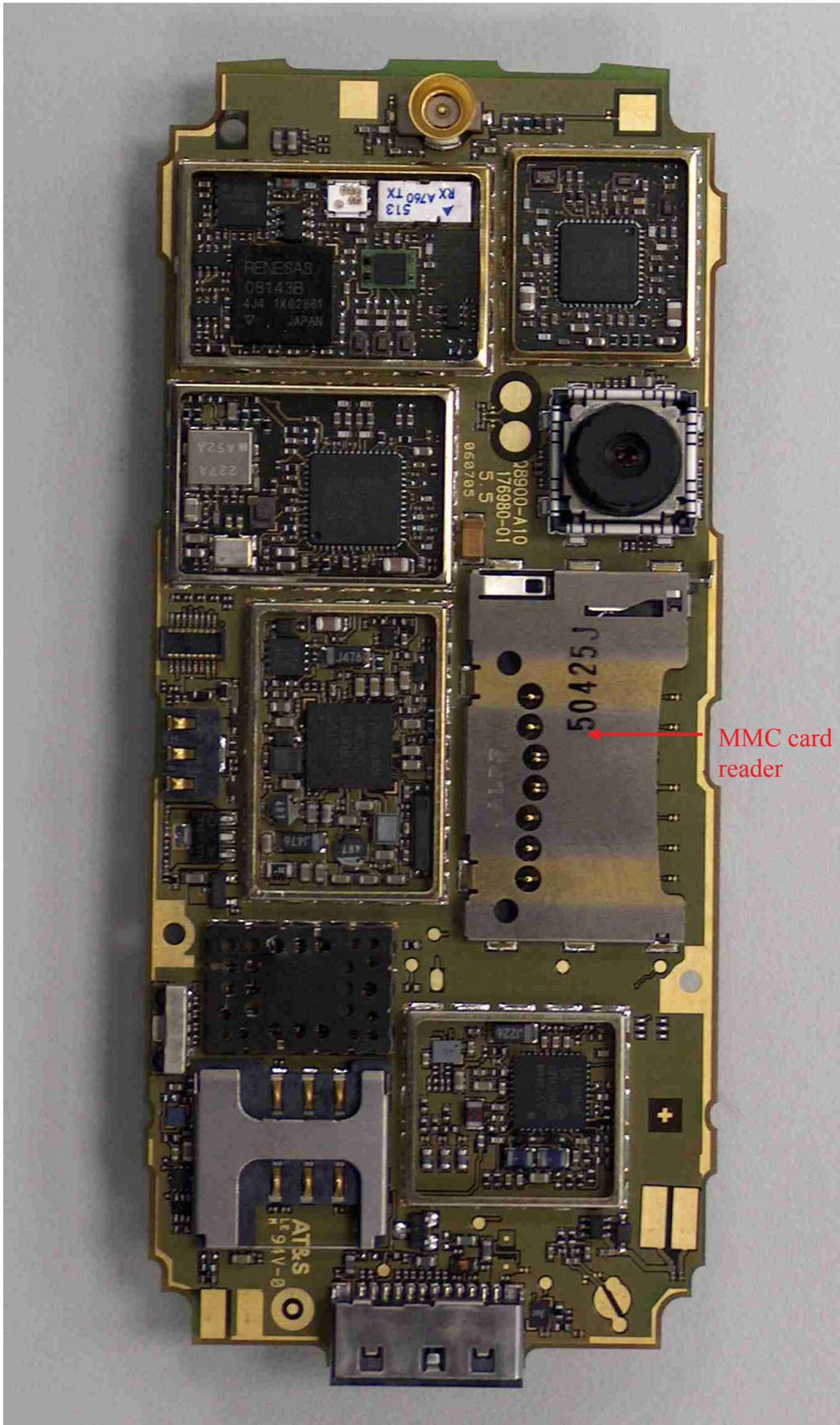
Figure 7 SXG75 PCB Back View Shields Removed
